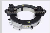
This is our new machine, stationary ring made by aluminum. Steel where strength is needed, aluminum where strength is less critical than weight.
