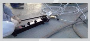
These high pressure hydraulic hand pumps are designed for high pressure hydraulic equipment. Its pressure is adjustable up to 40,600 psi, and customers can order also different size oil tanks for different applications. LAPP UK provides a wide range of accessories for this series, and these products are designed for high accuracy applications, and so are fully TUV certified.
